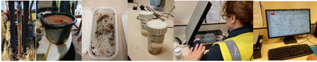
Figure 2: 1-Soil corer in barley field trial. 2-Washing machine. 3-Manual washing. 4-Clean root samples. 5-Root scanning. 6-Root analysis by WinRhizo.
